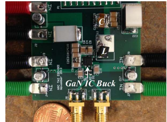
2.4 × 2.3mm integrated buck switching converter chip
